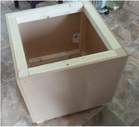
Use 9mm ply or MDF board for the sides. Two of the sides were 41 cm (W) x 30 cm (H) and the other two were 43 cm (W) x 30 cm (H). These are shown fixed in the image below. Each side panel is fixed using 4 screws.
