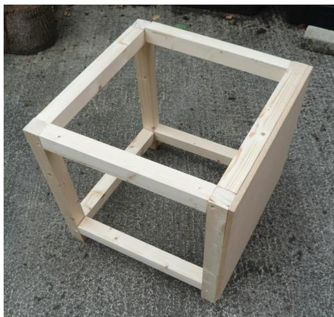
Build a frame for the stool using 34 x 34 mm smooth planed timber. The 4 vertical pieces are 35 cm long and the 8 horizontal struts are 34 cm long. They are screwed together as shown here. The 4 lower horizontal struts are fixed 5 cm from the end to form the feet for the stool. Only 1 screw is used for each joint as the whole structure tightens up when the side panels are fixed.
